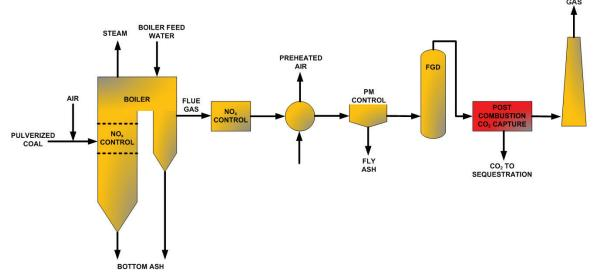
Figure 1. Schematic of PC Boiler Power Plant
