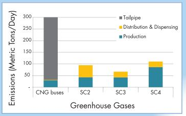
Figure 1. Well-to-wheel GHG Emissions for Different FCEB Scenarios
