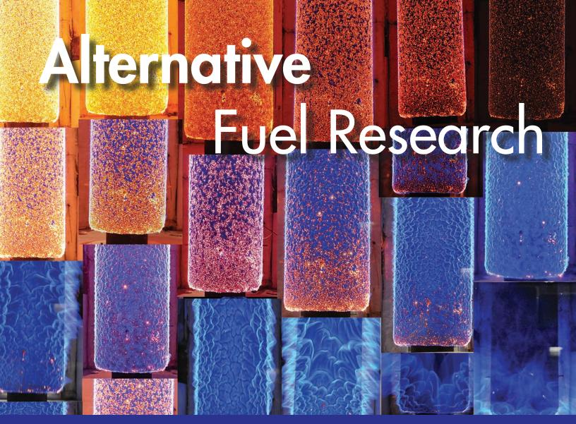
The Colors of Combustion. A wide range of visible spectrum colors observed during fuel flexibility experiments at the UCI Combustion Laboratory. The photo shows the structure of premixed flames with multiple fuel compositions and lean regime air to fuel ratios. Fuel compositions included blends of hydrogen, natural gas, and biogas. The ceramic Duratherm<sup>™</sup> burner by ALZETA Corporation uses a porous material to stabilize the reactions.
