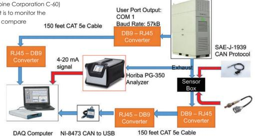
Figure 1: Flow Diagram of How Signals From Engine and Sensors are Sent to the DAQ Computer
