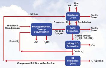
Figure 2: A Coal/Biomass Based IGFC Power Plant
