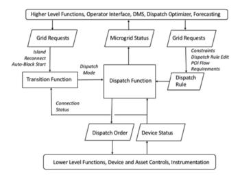
Figure 1: Master Microgrid Controller (MMC) Core Functions
