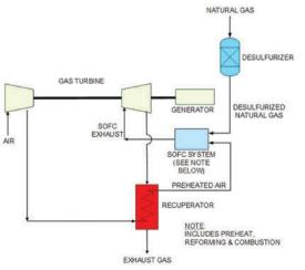
Figure 1: A Natural Gas Based SOFC/GT Hybrid
