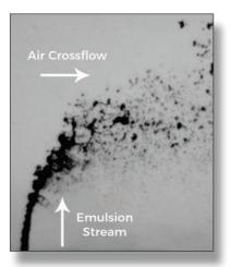
Figure 2. Liquid Jet in Crossflow
