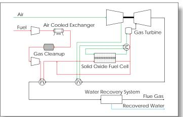
Figure 2. Fuel Cell - Gas Turbine Hybrid System
