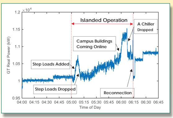
Figure 1. Gas Turbine Real Power Output
