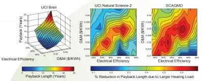
Figure 2: Payback period plot versus electrical efficiency and O&M for UCI Bren and the corresponding % difference in payback period due to larger heating load for UCI Bren compared to UCI Natural Science 2 (6.5 times larger heating load than Bren) and UCI Bren compared to SCAQMD (24 times larger). All buildings have a DG system sized to 50% of the maximum load, have 80% turndown, and cost \$2400/KW to install.
