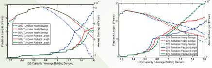
Figure 3: Impact of increased capacity on annual savings and payback for UCI Cal IT2. The system on the left has an electrical efficiency of 50% and O&M cost is \$0.01/KWh. The system on the right has an electrical efficiency of 25% and O&M cost is \$0.03/KWh Capital cost of DG was \$2400/KW
