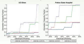
Figure 1: Capacity factor for a) UCI Bren and b) Patton State Hospital using economic strategy. Installed systems are sized to 50% of average building load. Patton State Hospital thermal demand is 34 times larger than UCI Bren
