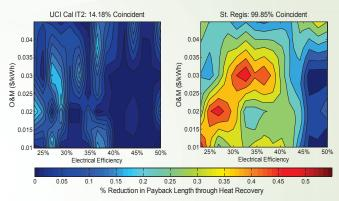
Figure 4: Percent reduction in payback due to waste heat recovery for UCI Cal IT2 and St. Regis. DG capital cost is \$2400/KW
