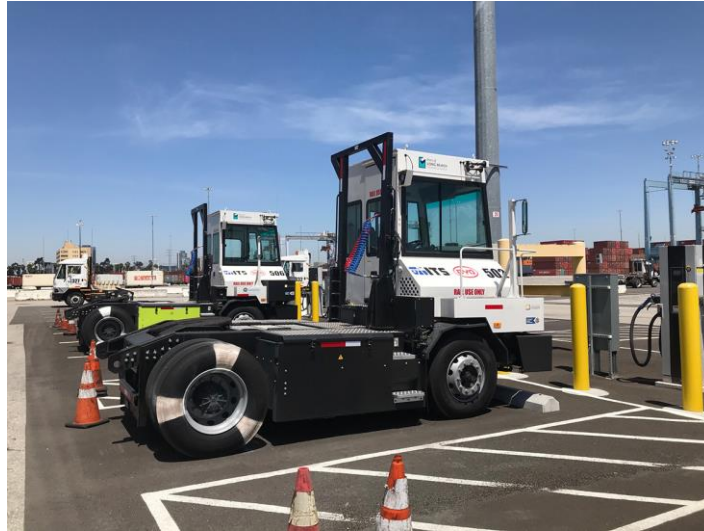
Figure 18. Battery-Electric Yard Tractor at POLB
