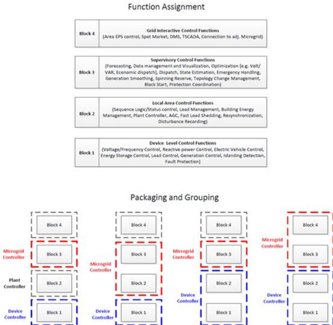
*Figure 2 Physical View of Microgrid Controllers*
