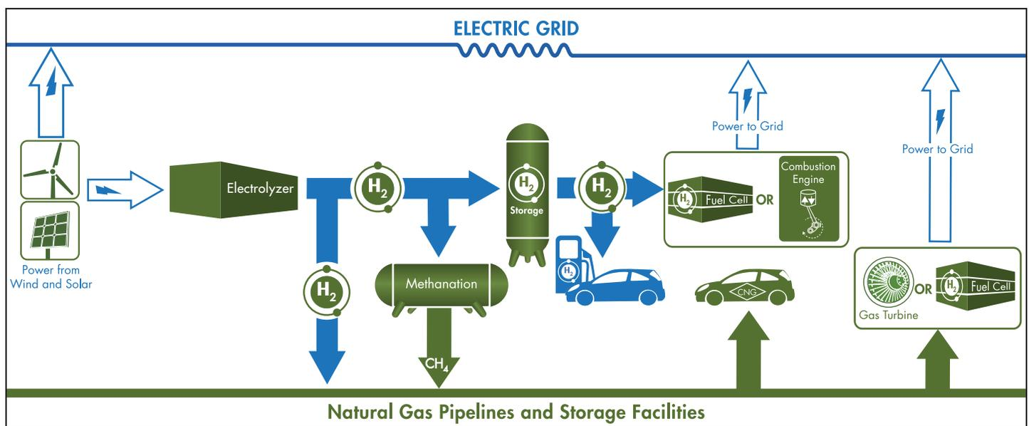
Figure 1. Power-to-Gas Concept
