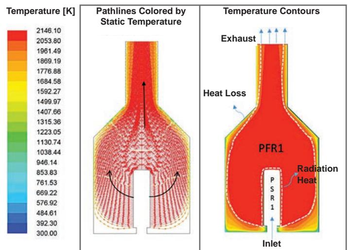
Figure 2. Associated CFD Simulation
