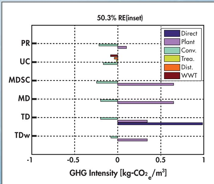
**Figure 1. Greenhouse Gas Intensity Change for Water Supply Infrastructure Components of Different Alternative Water Supply Methods at 50.3% Renewable Electricity.**
