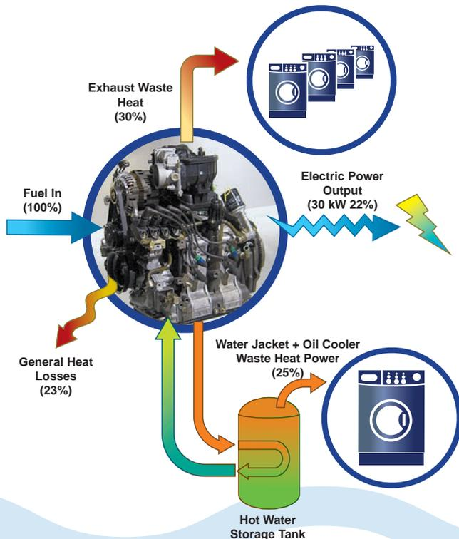
Figure 1. The Micro DG/CHP System
