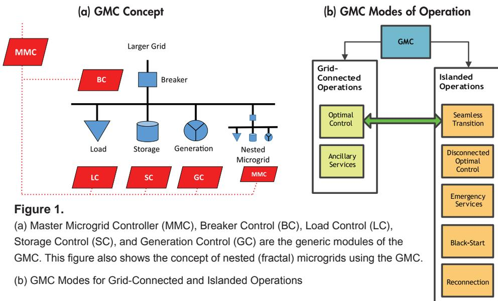
**Figure 1.** (a) Master Microgrid Controller (MMC), Breaker Control (BC), Load Control (LC), Storage Control (SC), and Generation Control (GC) are the generic modules of the GMC. This figure also shows the concept of nested (fractal) microgrids using the GMC. (b) GMC Modes for Grid-Connected and Islanded Operations
