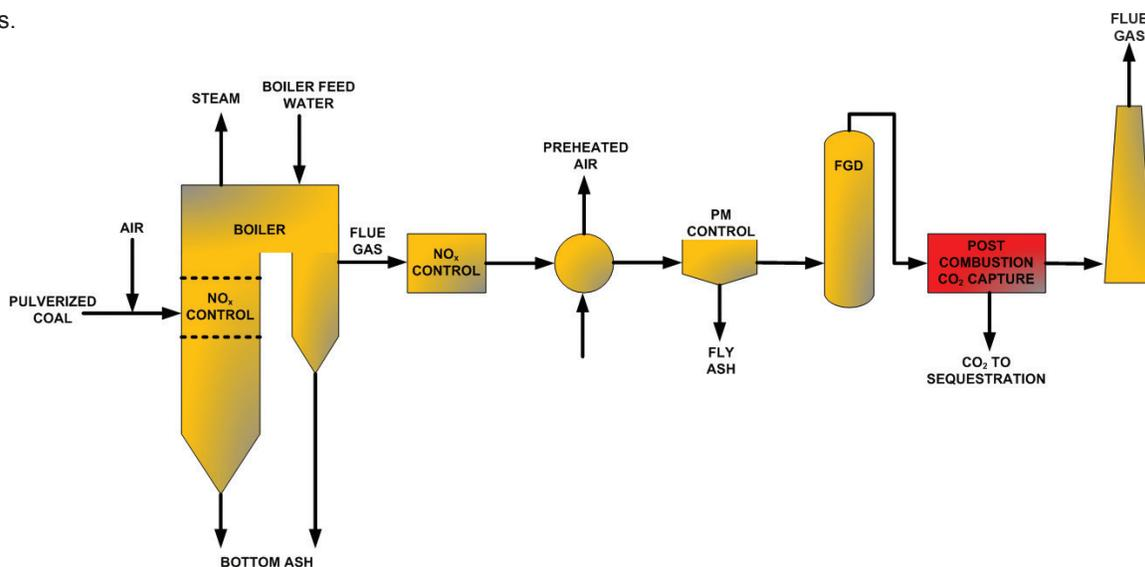
Figure 1. Schematic of PC Boiler Power Plant
