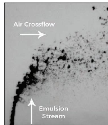
Figure 2. Liquid Jet in Crossflow
