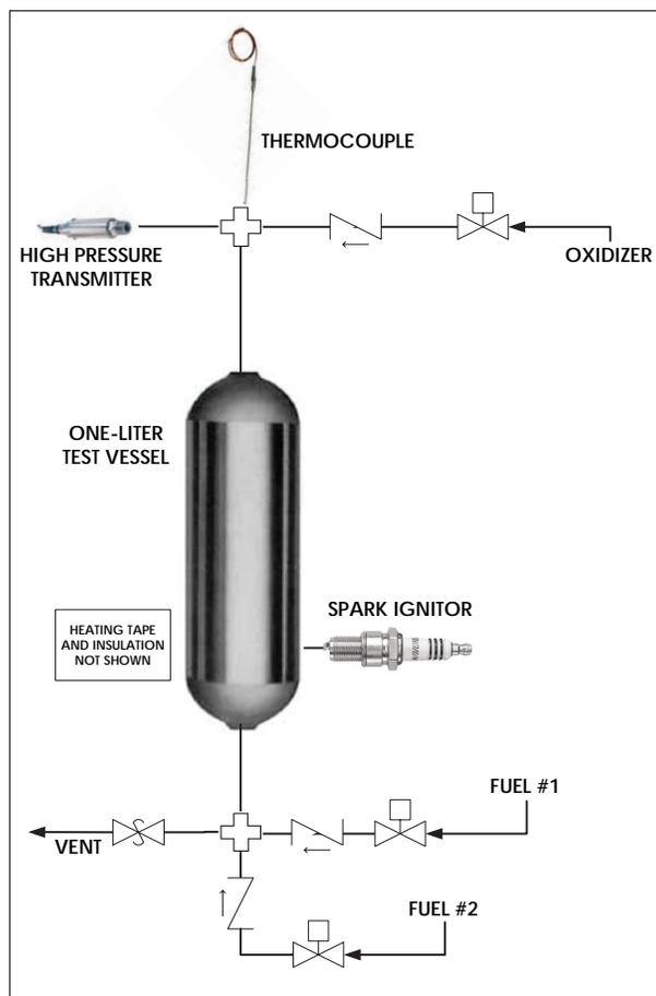
Figure 1. Schematic Diagram of UCICL Test Apparatus
