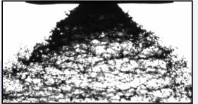
High Speed Exposure of Stable Emulsion Spray (0.689 MPa,  $\Phi$ = 0.28)
