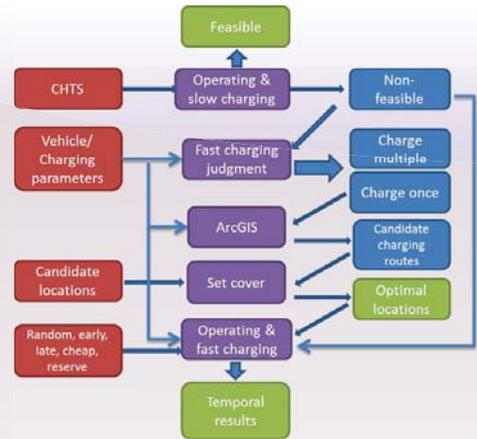
BEV Level 3 fast charging station allocation optimization model.
