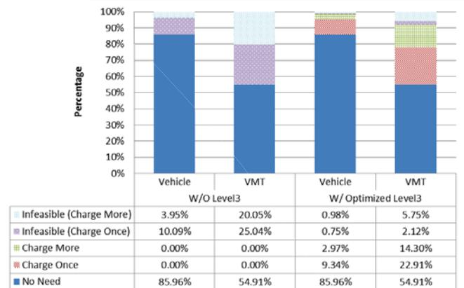
BEV and VMT feasibility with and without the optimized fast charging station network.
