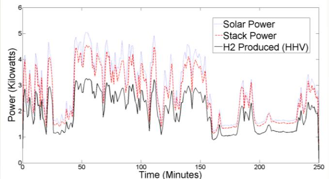
Direct electrical connection solar PV load following with 7kW PEM Electrolyzer System
