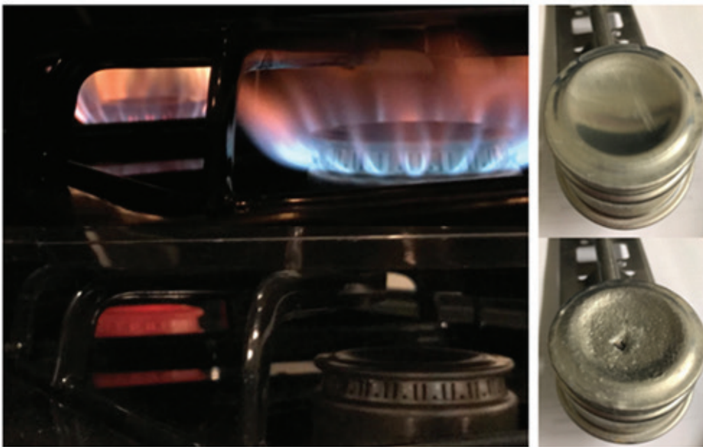
Figure 2. Cooktop Burner Before and After Flashback Due to Hydrogen Addition to Natural Gas
