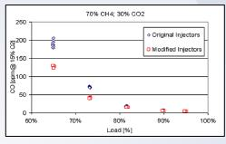
Figure 4: Injector comparison
