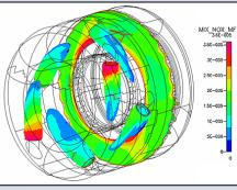
Figure 3. NO formation in combustor model
