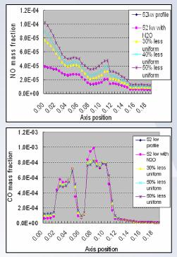
Figure 4. Average [NO] and [CO] along combustor centerline
