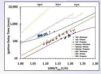
Figure 3: Comparison of chemical mechanisms to experimental ignition delay results
