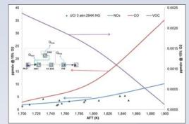
F3: Prediction of NOx, CO and VOC using CRN. Comparison with experimental NOx data at 3 atm.
