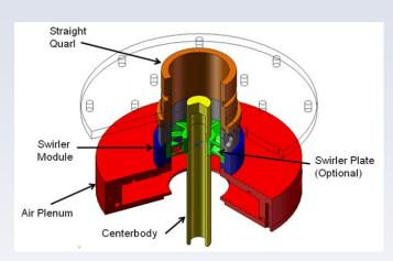
Figure 1. Modular Test Stand Sectioned View
