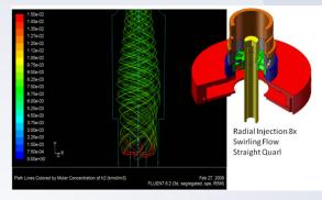
Figure 4. A path line originated from fuel injection port configures a radial injection with swirl.
